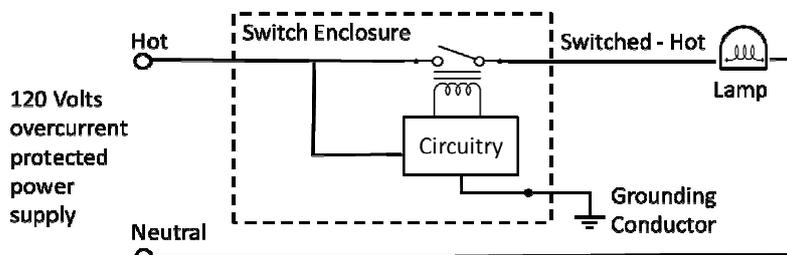
Figure 3 A simplified schematic of an electronic light switch using an equipment grounding conductor for the standby power supply.
