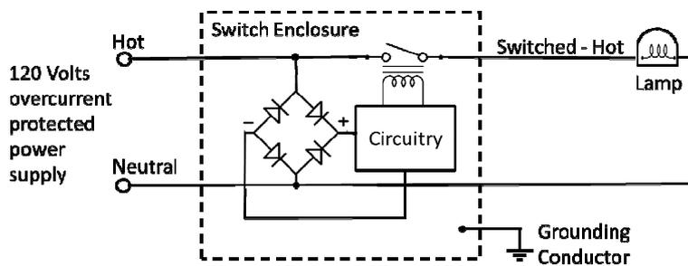
Figure 2 A simplified schematic of a light switch using a standby power supply installed according to Section 404.2(C) of the 2011 National Electric Code.
