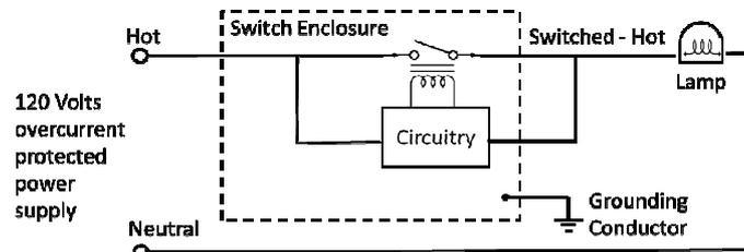
Figure 1 Standby power for electronic light switch passes through incandescent lighting assembly. The very low current passing through the lamps does not produce visible incandescence.
