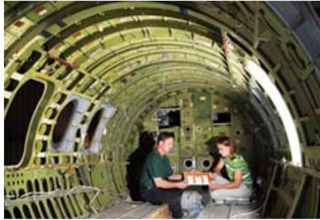
Figure 1 In the back of a commuter jet used as a testbed at Sandia, Dennis Roach and Ciji Nelson examine piezoelectric sensors placed on a printed circuit board for mounting to an aircraft structure.<sup>1</sup>
