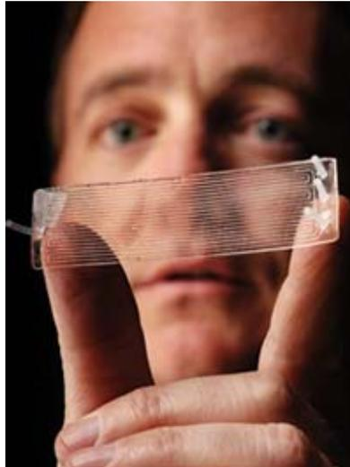
Figure 2 Dennis Roach with a Comparative Vacuum Monitoring (CVM) device showing galleries etched into the sensor's underside.<sup>2</sup>
