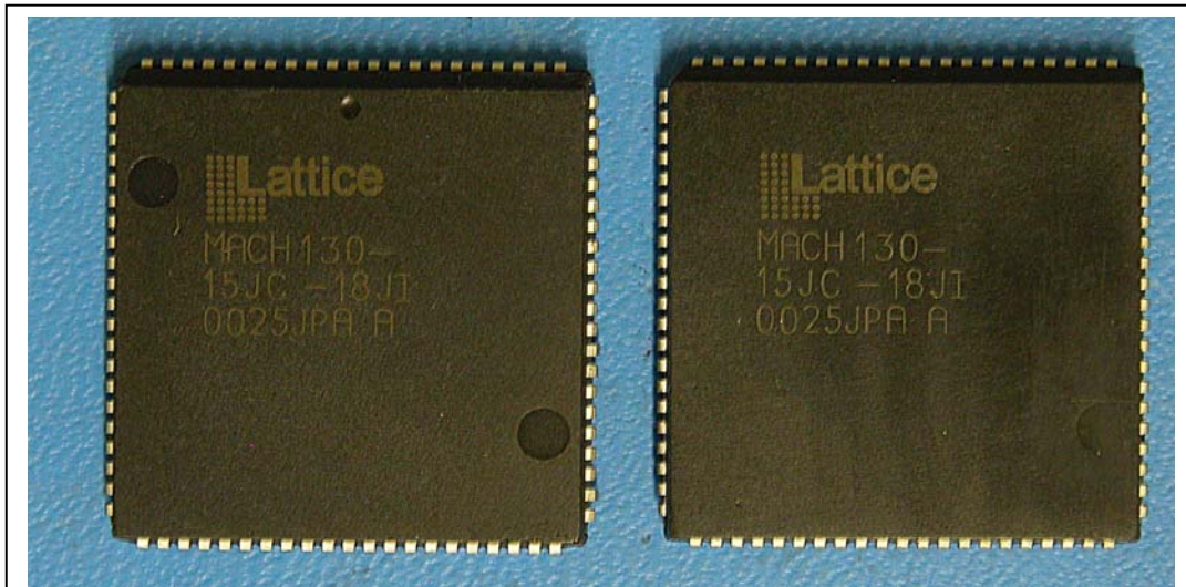
Figure 2: Sample with no Pin-1 marker, very odd. Notice both parts appear to be from the same date code and assembly lot, yet the one on the right is missing the pin-1 dimple and most of the mold marks. Lighting has been adjusted to enhance the markings.
